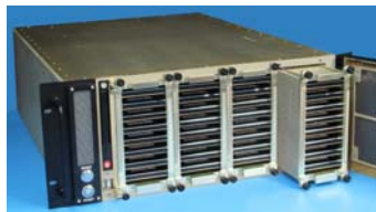
Figure 2. Chassis View showing one QuickPac canister partially withdrawn.
