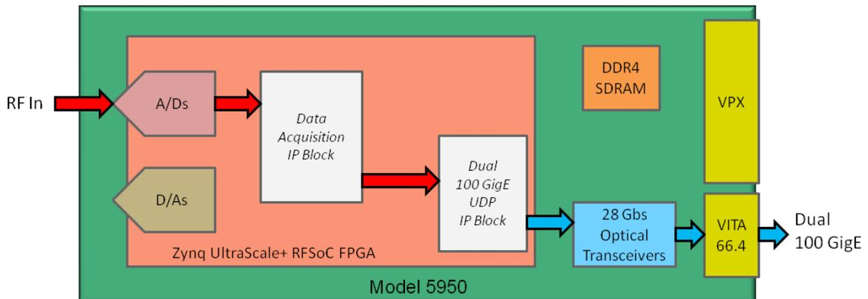
**Example Application 3 - Waveform and Radar Chirp Generator**
